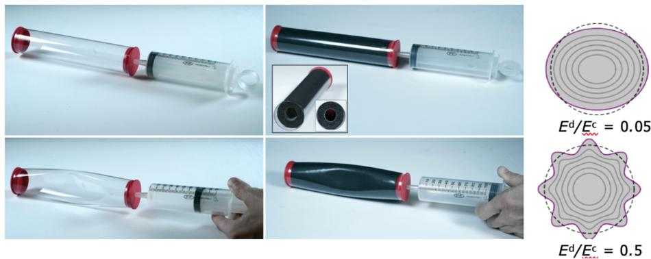
Figure 1: Buckling induced by pressure on an empty thin cylindrical shell (left) and on a shell enclosing a material (middle). The different ratio between Young's modulus of the disk ( $E^d$ ) and of the coating ( $E^c$ ) produces various bifurcation patterns which can be different from the mere oval modes of rings (right).
