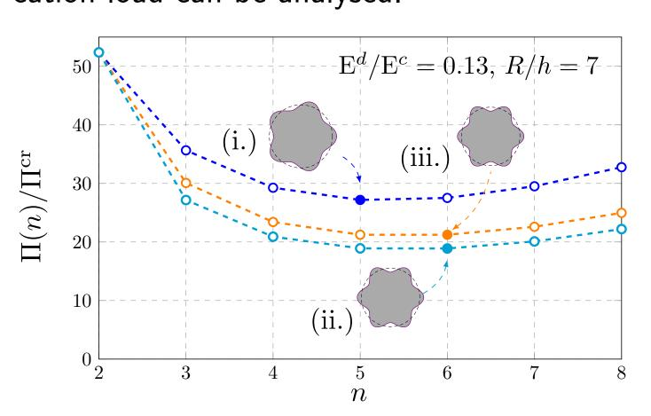
The critical value corresponds to the integer number n that minimises the equation The presence of the inner disc may lead to the predominance of high-wavenumber modes. Once a value of n, corresponding to a given applied pressure  $\Pi(n)$ , is fixed, the Kolosov–Muskhelishvili formulae allow for the determination of all elastic fields at every point within the boundary of the disc.
