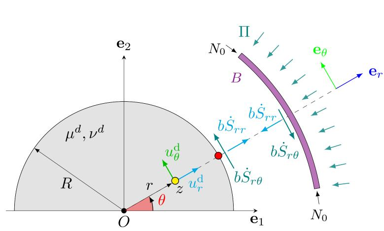
At bifurcation, a non-trivial incremental deformation occurs, causing the disc to experience incremental stress and strain. The resulting incremental traction at the disc's boundary, multiplied by its thickness b, gives rise to an incremental force acting on the rod.
