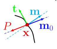
The load is said to be a "dead" radial load if it remains parallel to the normal unit vector  $\mathbf{m}_0$ when passing from the reference to the current configuration.
