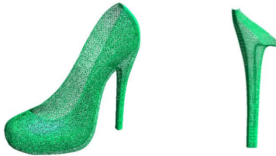
Figure 1: Finite element model of a shoe and a high heel.
