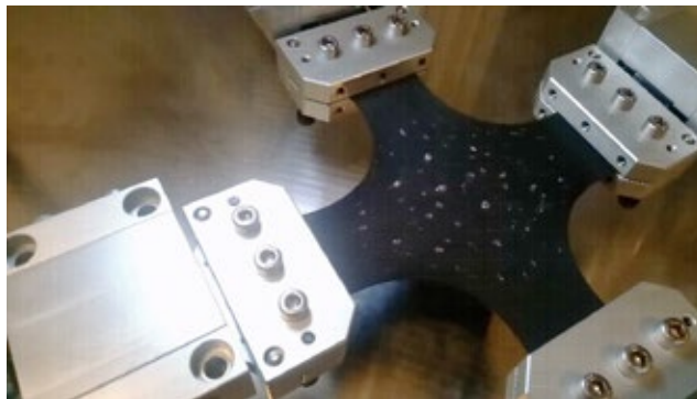
Figure 1: Biaxial test on cruciform specimen. The optimal shape design is validated with an in-house tensile machine. The white spots on the specimen constitute the speckle pattern used for image processing and full field measurements.
